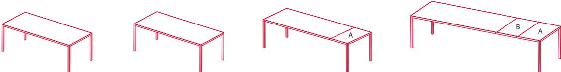
According to the customer's needs, the nominal length of the table can be increased from 19.68" (A) to 39.37" (A+B).
